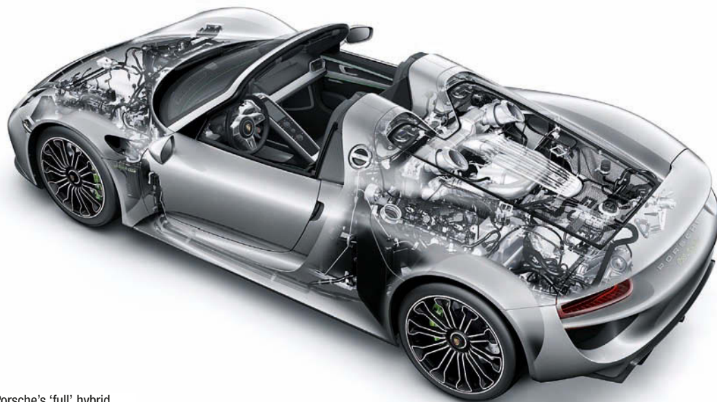
Porsche's 'full' hybrid design means the car can travel purely using electric power...
